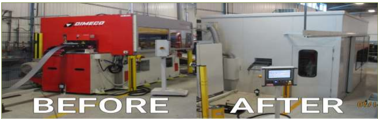
Figure 5.6 The above picture shows how a noisy machine has been encased to reduce the noise 11
